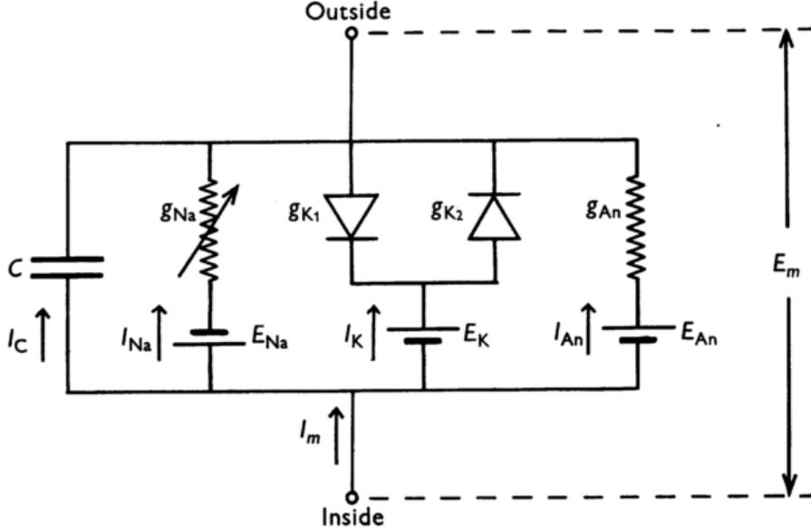
Figure 5: Diagram of the circuit from Noble's 1962 paper
