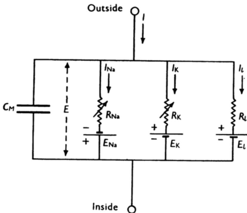
Figure 3: Diagram of circuit from Hodgkin & Huxley’s paper
